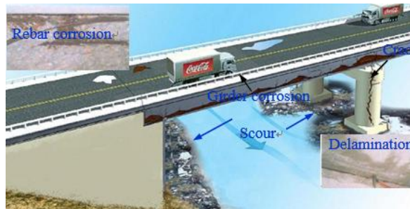
Figure 1.1. Schematic view of various structural behaviors.
